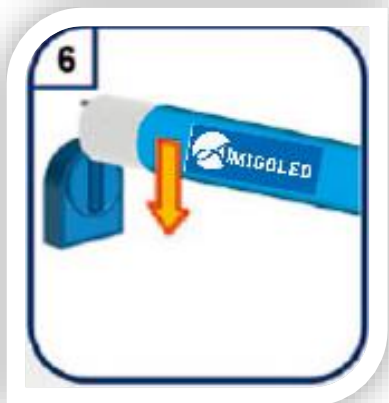
Insert the LED lamp into the lamp holder.
