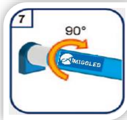
Secure the position by turning the lamp by 90° .
