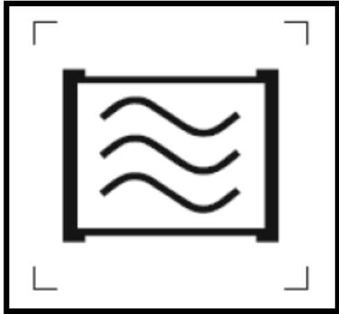
Lamp suitable for Electronic Ballast
