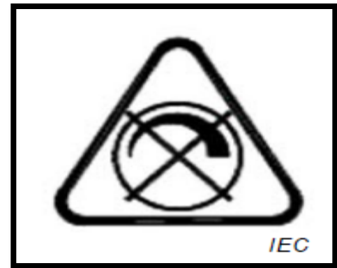
Lamp not suitable for emergency operation
