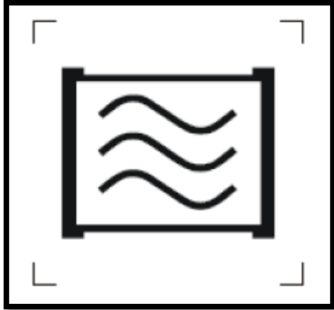
Lamp suitable for Electronic Ballast
